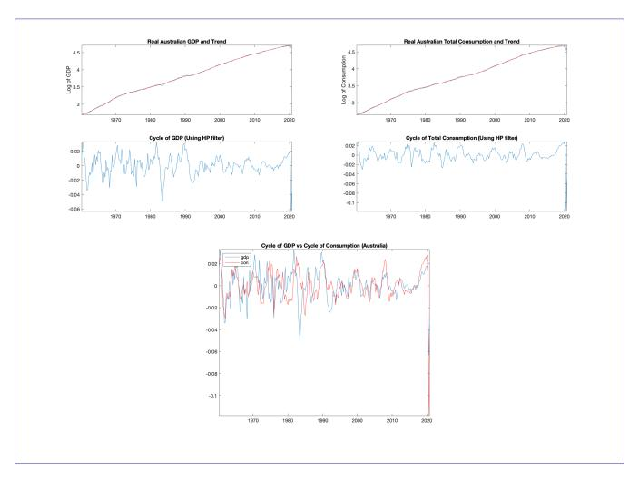
(b) For the cycle of each variable compute the standard deviation, the correlation with the output, and the autocorrelation.
